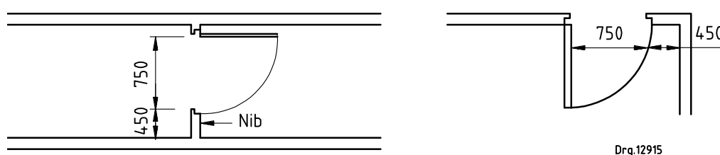
Figure 8 — Doorways in restricted spaces
