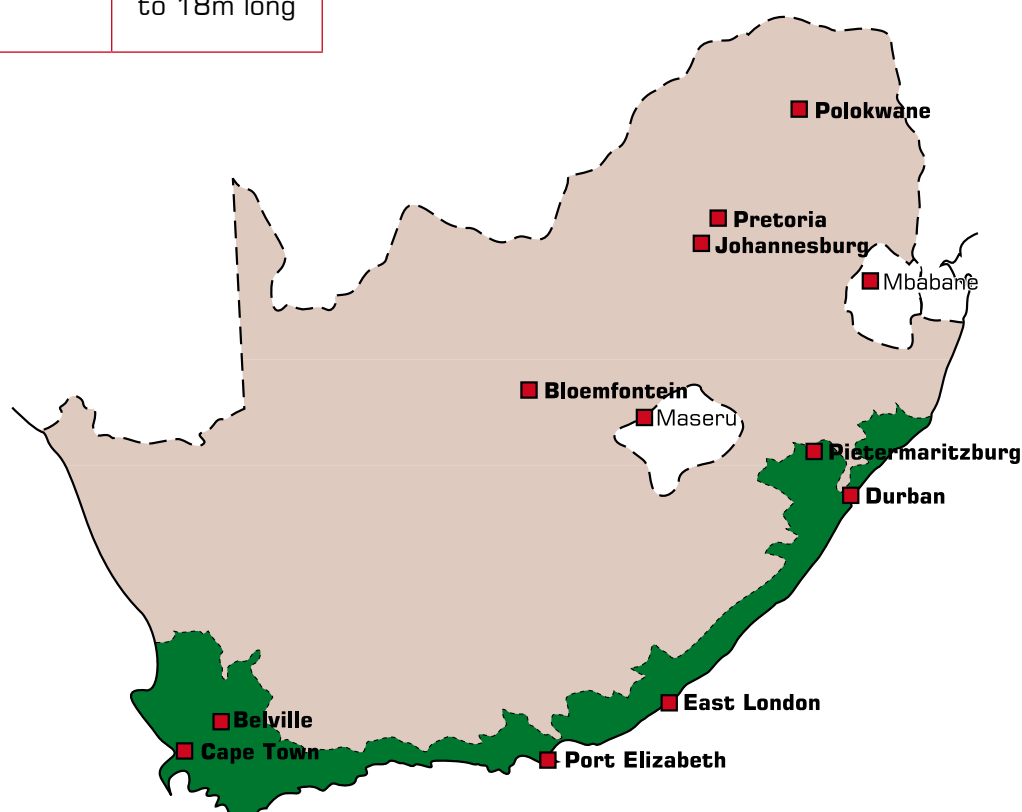
Figure 1: Map of South Africa showing coastal and other areas (shaded) currently requiring treatment of structural South African pine against biological attack
