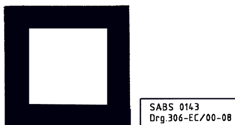
Fig. 19 — Elements cut by the Section
