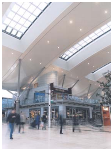
Above - The Chimes Shopping Centre, Uxbridge. Colt worked closely with the design team and the contractors Costain Skanska Joint Venture, on the design and installation of the smoke ventilation system which included 88 Colt glazed natural Kameleon ventilators and 6 trapezoid shaped glazed natural double flap Meteor ventilators.
