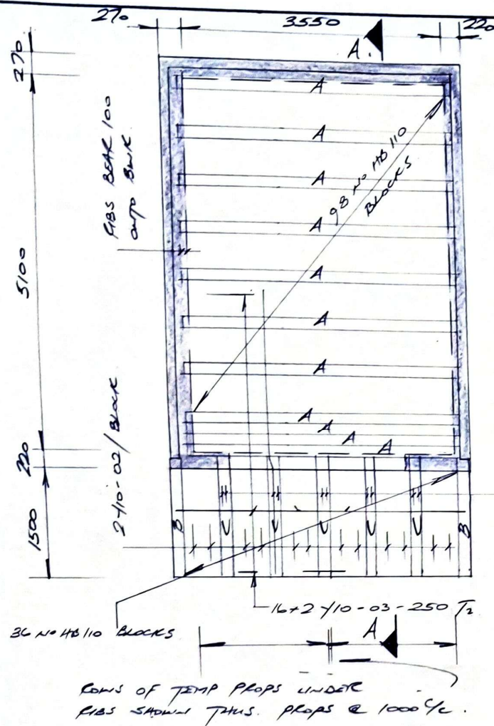
PLAN SHOWING 170/205 THICK RIB & BLOCK SLAB. (1:50)
