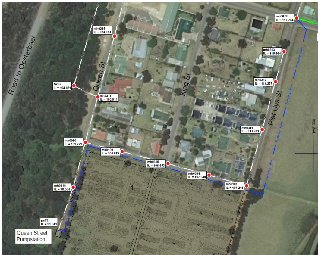
Figure 4: Existing pumpstation and rising main
