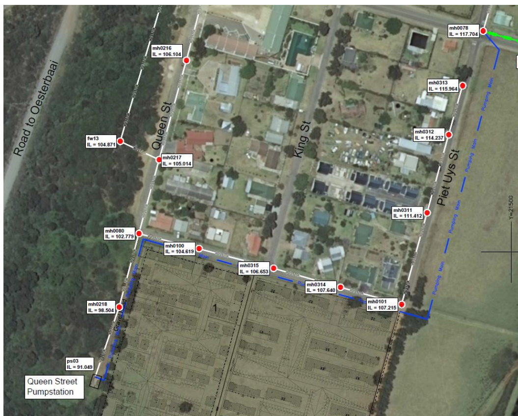
Figure 4: Existing pumpstation and rising main
