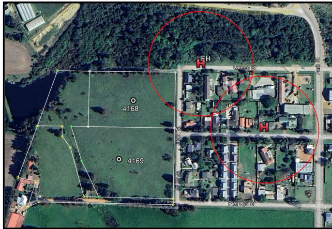
Figure 6: Existing Fire hydrants
